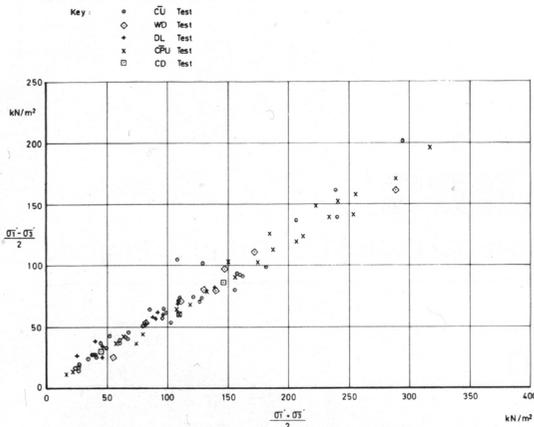
Figure 11. Summary of triaxial test failure stresses - decomposed volcanics
