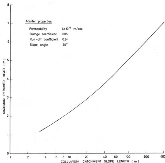
Figure 5. Maximum perched head over base of colluvium (1 in 10 year)
