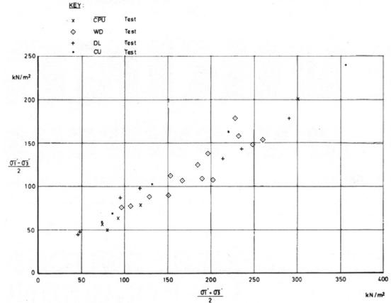
Figure 12. Summary of triaxial test failure stresses - decomposed granite
