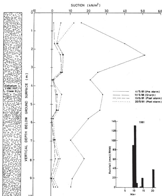
Figure 6. Suction response to storm 10/5/81 to 12/5/81 Chater Ridge - Caisson K3 - Instrument Group E/2/227
