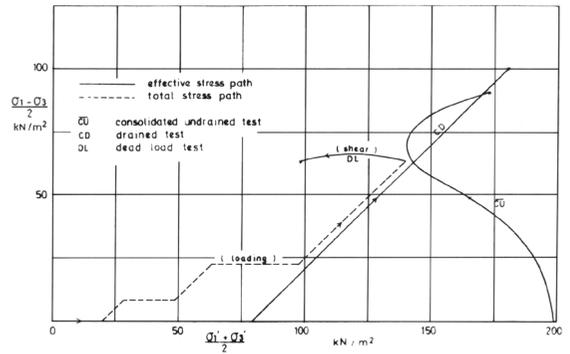
Figure 8. Typical colluvium saturated triaxial test stress paths
