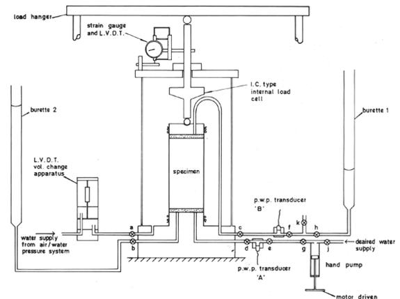
Figure 7. Dead load test apparatus
