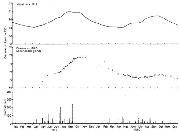
Figure 3. Comparison of groundwater model with Piezometer OH1B
