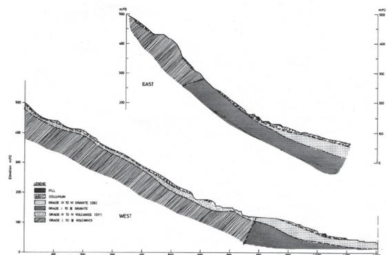
Figure 2. Typical geological cross sections
