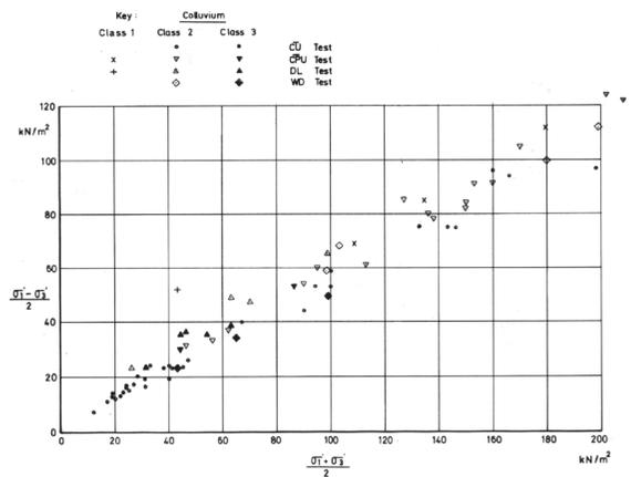
Figure 10. Summary of triaxial test failure stresses - colluvium
