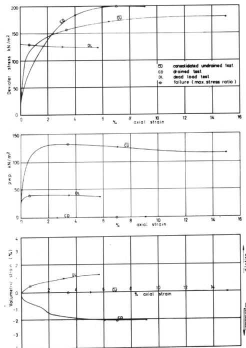
Figure 9. Typical colluvium saturated triaxial test stress - strain plots (shearing stage)
