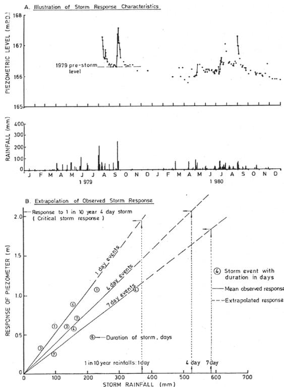
Figure 4. Extrapolation of storm response
